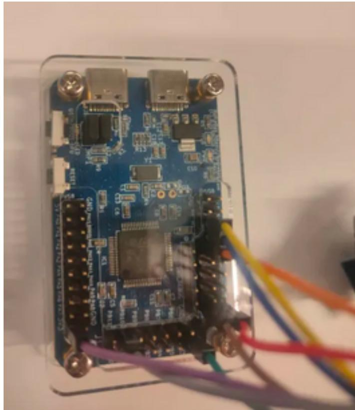
**Figure 50:** Top view of Hydrabus wiring
