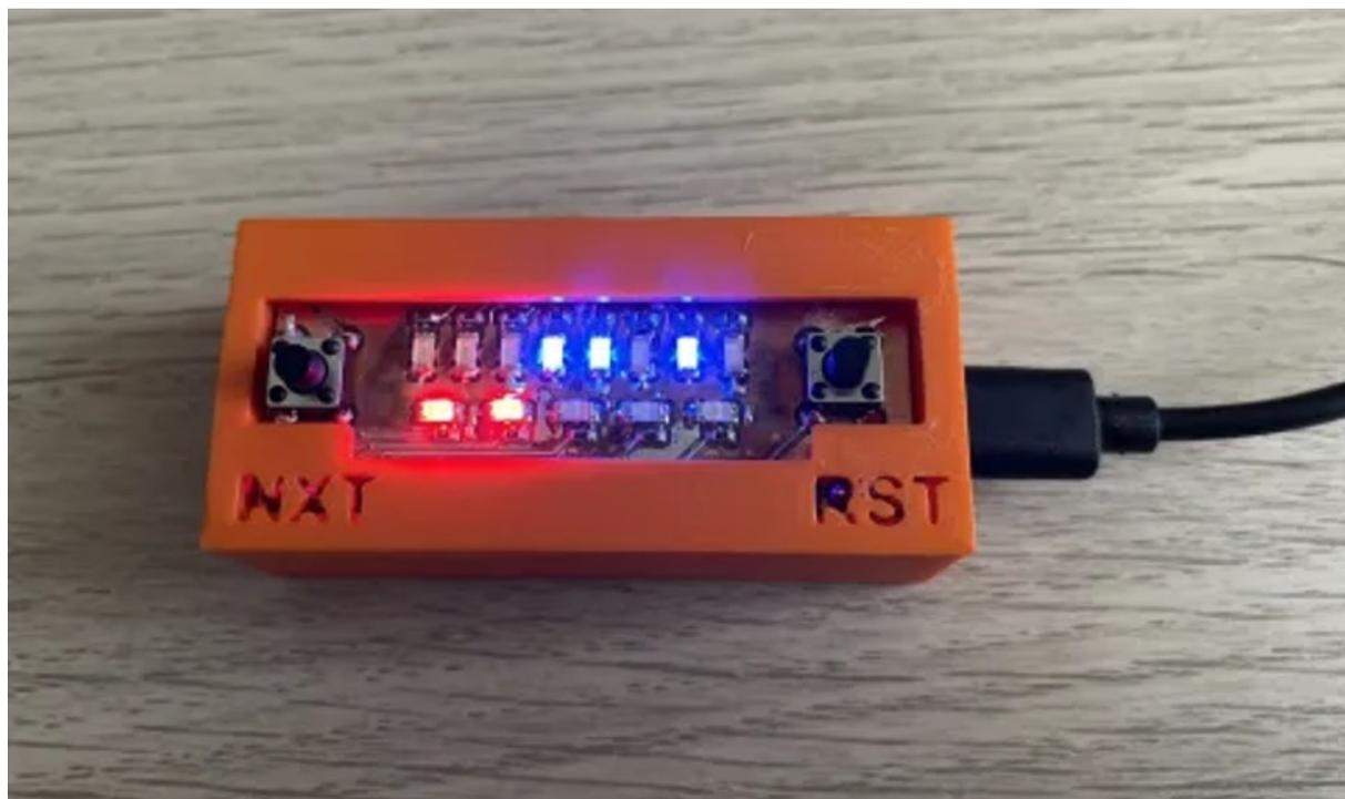
Interacting with the device was simple: it had a RESET button and a NEXT button. Pressing NEXT caused the LEDs to flash, while RESET initiated a cool animation with the LEDs flashing. Each press of NEXT revealed a different state. Quickly, we understood that the lower 5 red LEDs indicated the current state number, giving the clue of a total of 32 different deterministic states. But how would it reveal a flag? Link to video: [YouTube](#).
