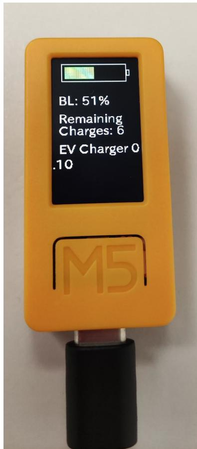
**Figure 37:** Operational M5StickC device with challenge program
